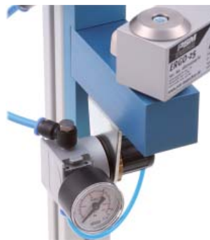
Air pressure regulator adjusts vertical lift force of the arm
