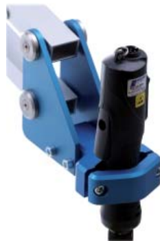
Universal tool fixture accepts up to 1.57 in. diameter tool
