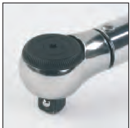
72 tooth reversible ratchet gives a narrow 5° engagement angle.
